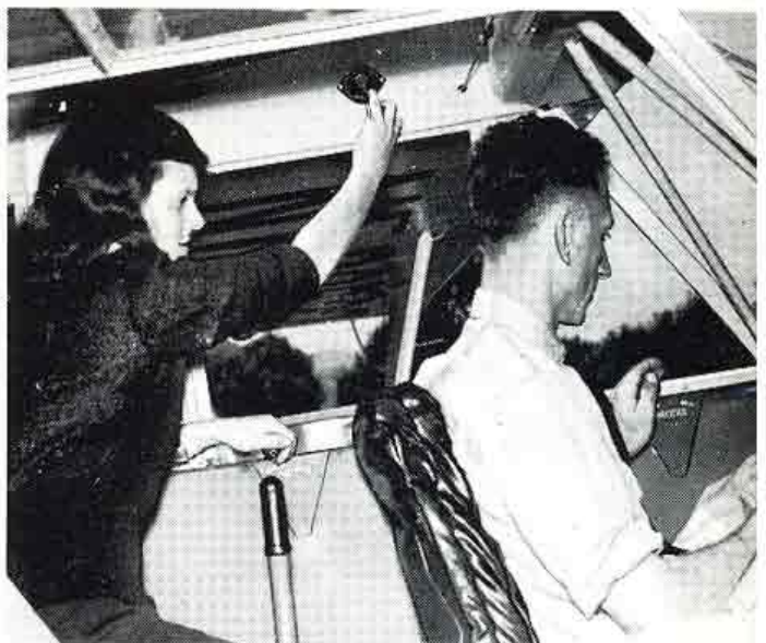
16. Near end of runway stop, apply brakes, advance throttle to 1400 RPM and check the magnetos with the tachometer. Check for other aircraft landing or taking off. If clear, proceed to position on runway.
