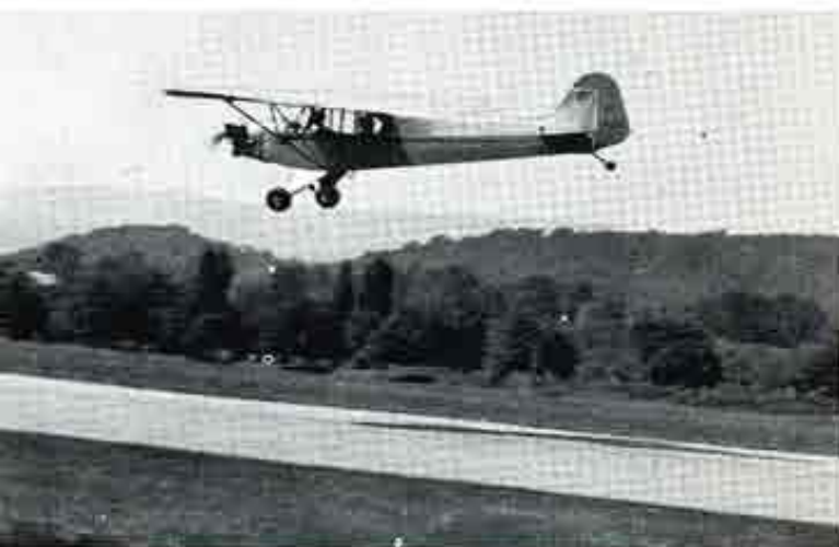
49. When ship is about 15 feet above runway, slowly start to apply back pressure on stick to break glide.
