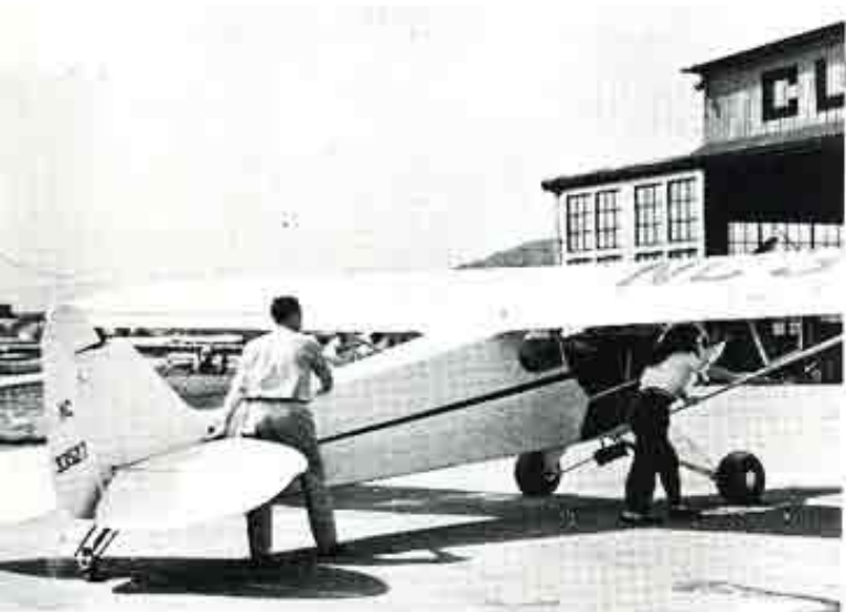
53. Turn off switch, advance throttle full forward, then close throttle. Get out of plane and push it into hangar.
