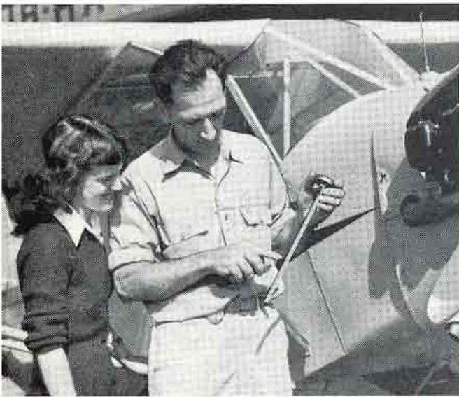
3. Check the oil by removing the cap and looking at the oil stick.
