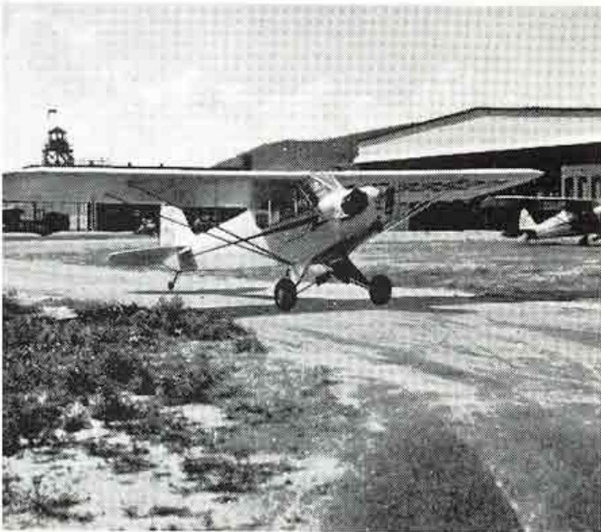
15. Observe the windsock and S-taxi to the runway. Always take off and land INTO the wind. Do not taxi faster than normal walking speed. Look around and ahead constantly for other aircraft.
