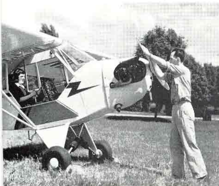
11. Now the prop is swung through to start engine.
