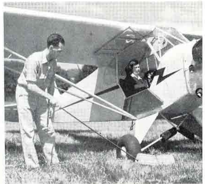
12. The chocks are pulled from in front of the wheels, using the ropes attached to them.
