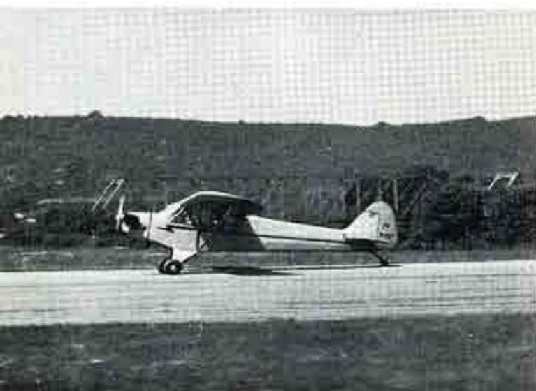
51. As flying speed is lost, ship will settle to ground in three-point position.
