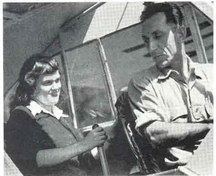
6. Check rudder and stick controls for freedom of movement by moving them in all positions.
