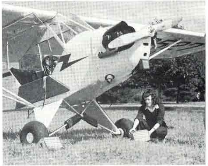
4. Place chocks securely in front of both wheels.
